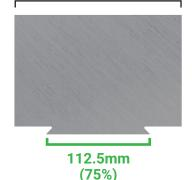
We recommend dovetail width should not be **less than** 75% of the width of the stock.
