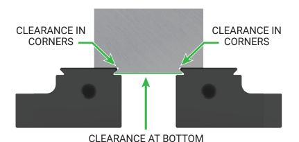
When a **proper** dovetail is used, jaw/dovetail fixture **acts** as a **wedge** trying to split the material in the corner.
