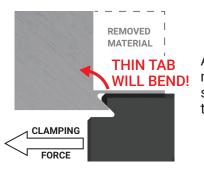
A thin tab and/or insufficient material on the top locating surface will allow the part to move during machining.
