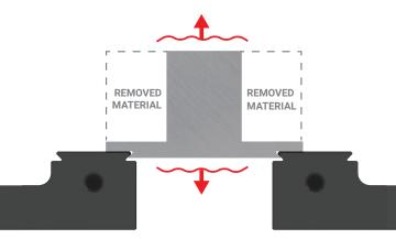
Even though this part has tabs thick enough to prevent breaking, the dovetail is not properly positioned under the part. This may result in excessive vertical vibration.
