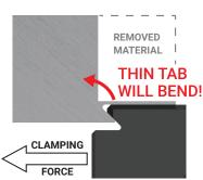
A thin tab and/or insufficient material on the top locating surface will allow the part to move during machining.
