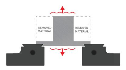
Even though this part has tabs thick enough to prevent breaking, the dovetail is not properly positioned under the part.
