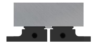
Excessively narrow dovetail will concentrate support at the center of the stock and potentially cause chatter.
