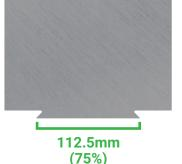
We recommend dovetail width should not be **less than** 75% of the width of the stock.
