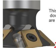
This issue is caused when dovetail cutter inserts / flutes are worn or broken.
