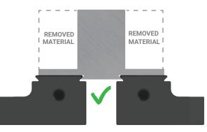
For narrow parts, position the dovetail as close as possible to the **finished part's** center of mass.
