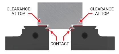
Locating on bottom step causes material to become a wedge trying to split the jaw. **This can break the jaw!**
