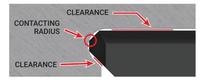
An overly wide inside corner radius allows material to contact the corner of the jaw, preventing it from locating correctly.
