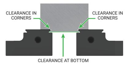
When a proper dovetail is used, jaw/dovetail fixture acts as a wedge attempting to split the material in the corner.
