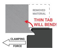
A thin tab and/or insufficient material on the top locating surface will allow the part to move during machining.
