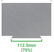
Dovetail width should not be less than 75% of the width of the stock.
