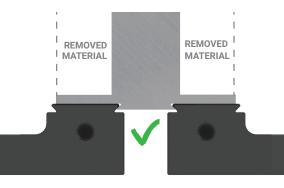
For narrow parts, position the dovetail as close as possible to the finished part's center of mass.
