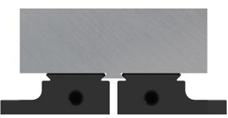
Excessively narrow dovetail will concentrate support at the center of the stock and potentially cause chatter.
