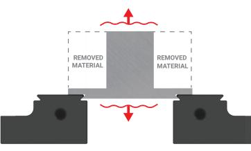
Even though this part has tabs thick enough to prevent breaking, the dovetail is not positioned correctly under the part. This may result in excessive vertical vibration.
