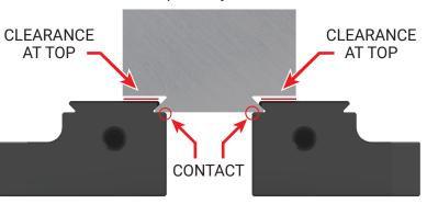
Locating on bottom step causes material to become a wedge trying to split the jaw.
