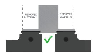
For narrow parts, position the dovetail as close as possible to the finished part's center of mass.
