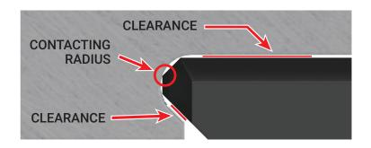
An overly wide inside corner radius allows material to contact the corner of the jaw, preventing it from locating correctly.
