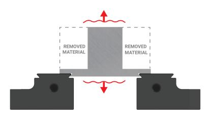
Even though this part has tabs thick enough to prevent breaking, the dovetail is not positioned correctly under the part. This may result in excessive vertical vibration.
