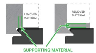
If more support is needed, decrease dovetail width or increase tab thickness.
