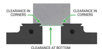
When a proper dovetail is used, jaw/dovetail fixture acts as a wedge corner.
